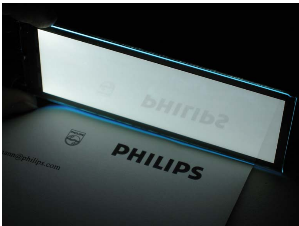
Caption: White small molecule OLED measuring 4 by 12 cm 2 (Picture by Philips Lighting)
